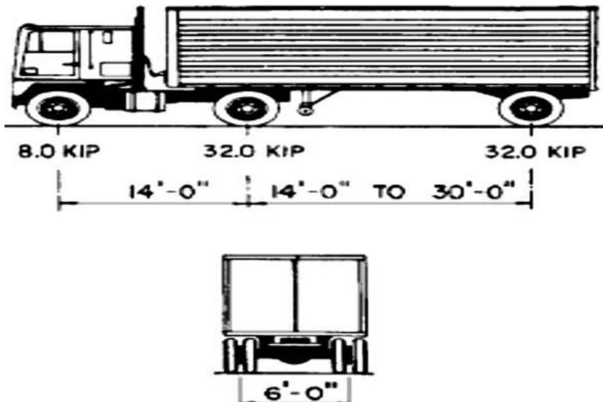
**Fig. 2.4 Characteristics of Design Truck**
