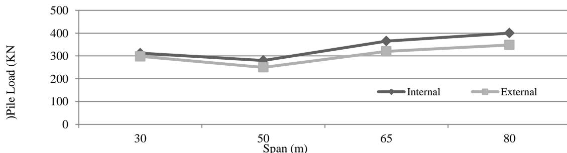
Fig. 3.11 Pile Load for Internal and External Prestressing Systems
