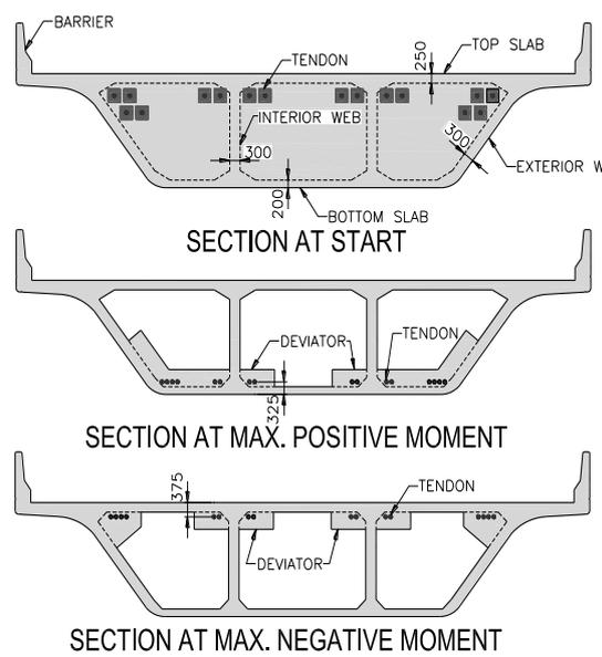
Fig. 2.3 Box Girder with External Tendons
