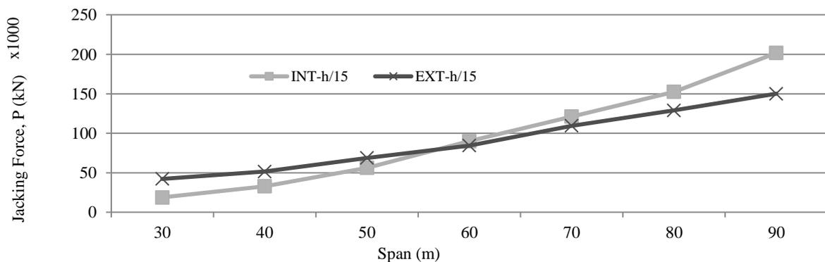
**Fig. 3.4 Req. Jacking Force for Int. & Ext. Box Girders, Span to Depth ratio, L/h=15**
