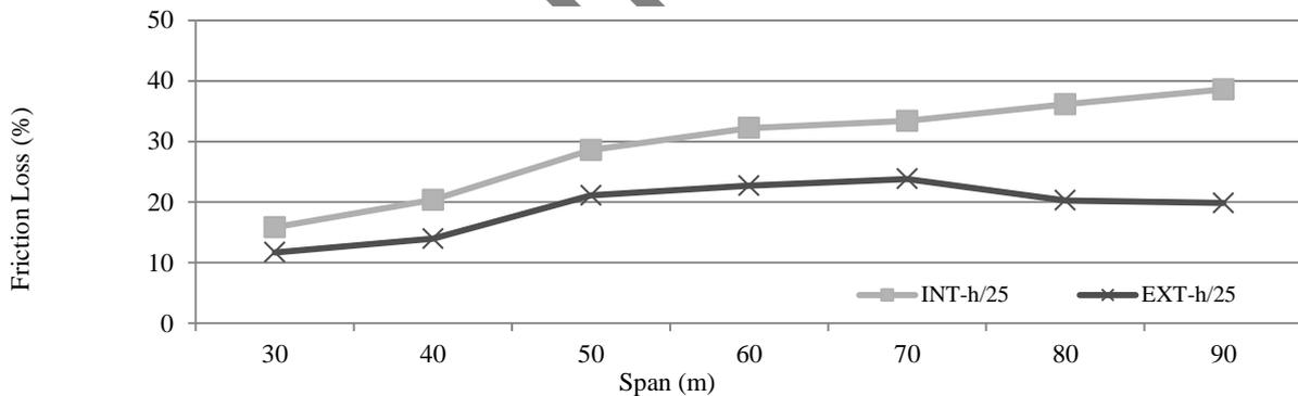
**Fig. 3.3 Friction Losses for int. & ext. Box Girders, span to depth ratio, L/h=25**
