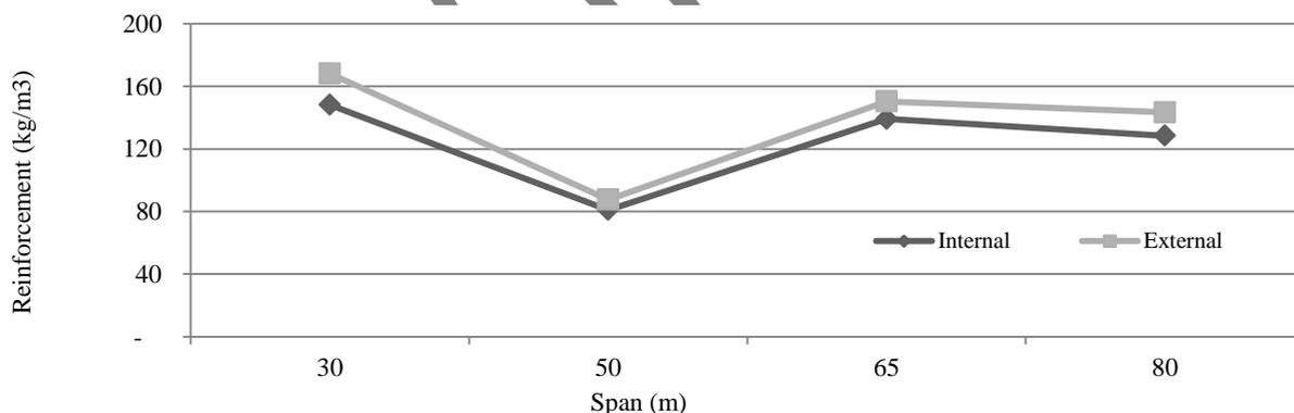
**Fig. 3.13 Pilecap Reinforcement for Internal and External Prestressing Systems**
