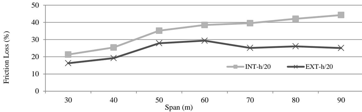
**Fig. 3.2 Friction Losses for Int. & Ext. Box Girders, span to depth ratio, L/h=20**
