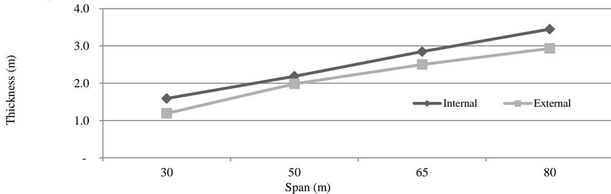
**Fig. 3.12 Pilecap Thickness for Internal and External Prestressing Systems**
