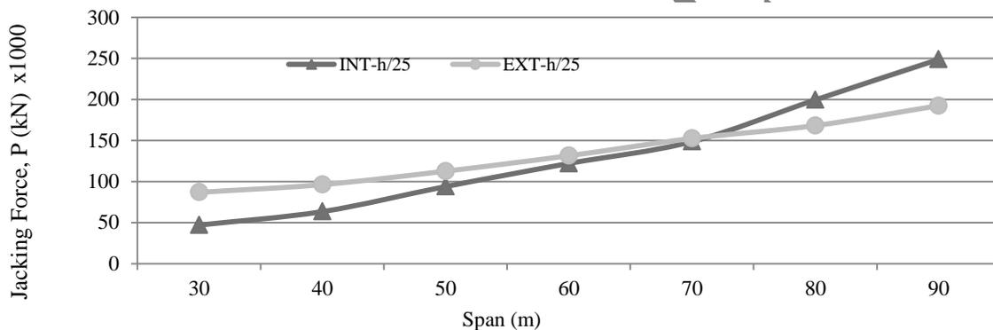
**Fig. 3.6 Req. Jacking Force for Int. & Ext. Box Girders, Span to Depth Ratio, L/h=25**
