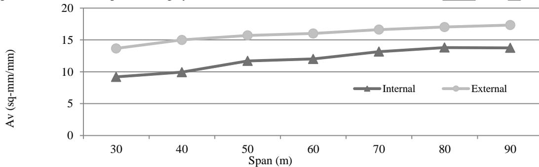
Fig. 3.9 Required Web Shear Reinforcement for int. & ext. Prestressing Systems
