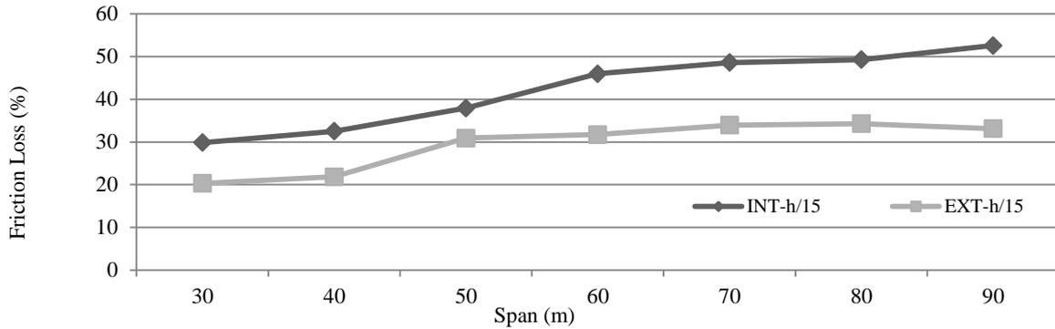
**Fig. 3.1 Friction Losses for Int. & Ext. Box Girders, span to depth ratio, L/h=15**
