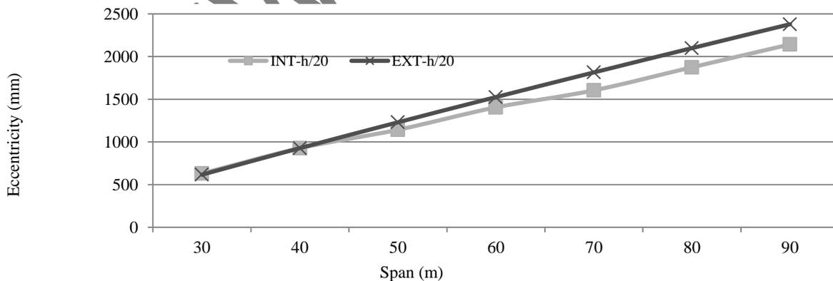
**Fig. 3.7 Eccentricity Variation for Int. & Ext. Girders with Span to Depth Ratio, L/h=20**
