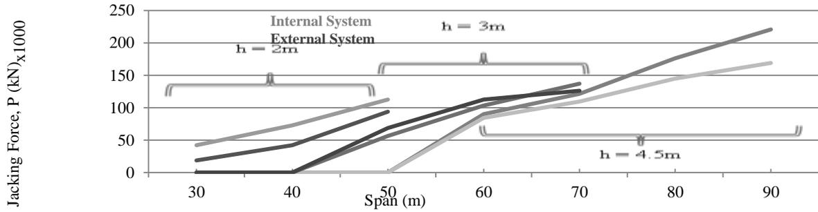
Fig. 3.8 Influence of Girder Depth on Required Amount of Prestressing
