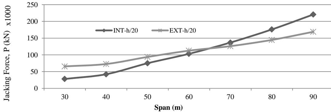
**Fig. 3.5 Req. Jacking Force for Int. & Ext. Box Girders, Span to depth ratio, L/h=20**
