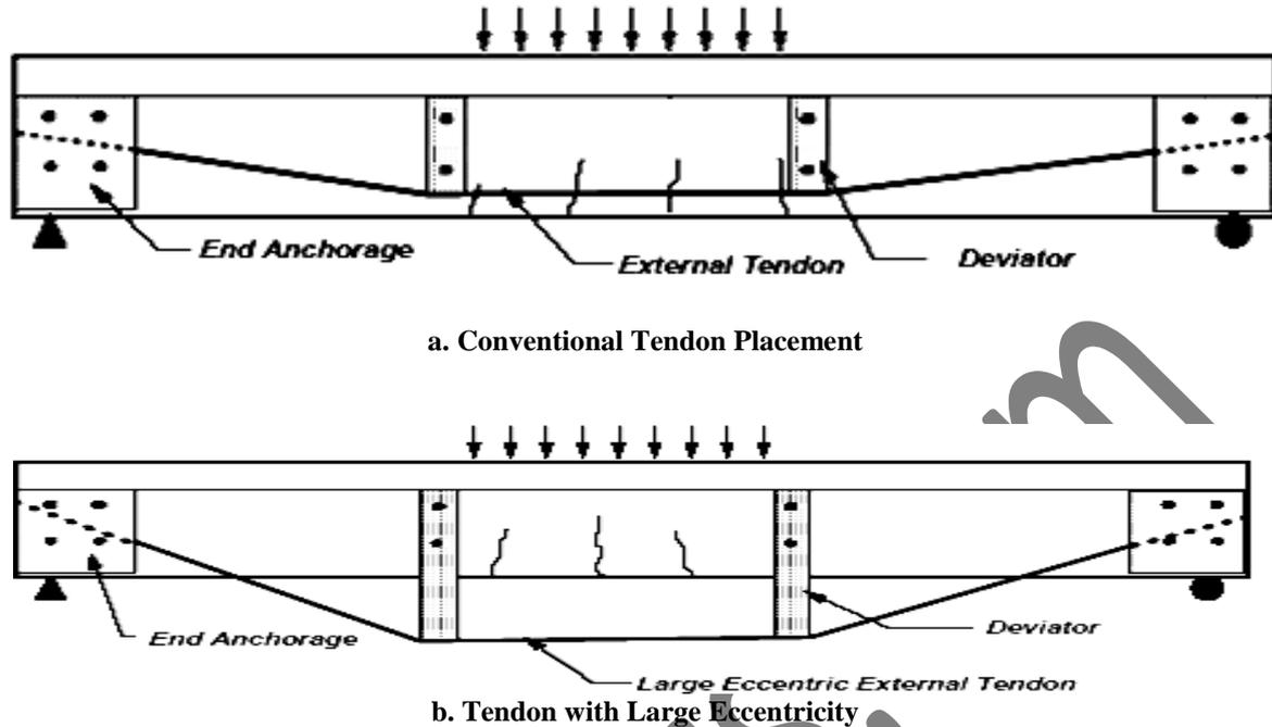
Fig. 1.3 Possible Tendon Placement in External Post-Tensioning
