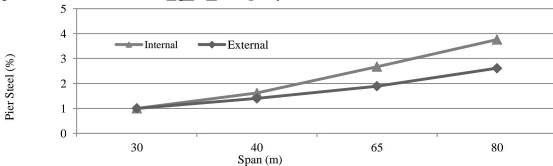
Fig. 3.10 Required Pier Reinforcement for int. & ext. Prestressing Systems
