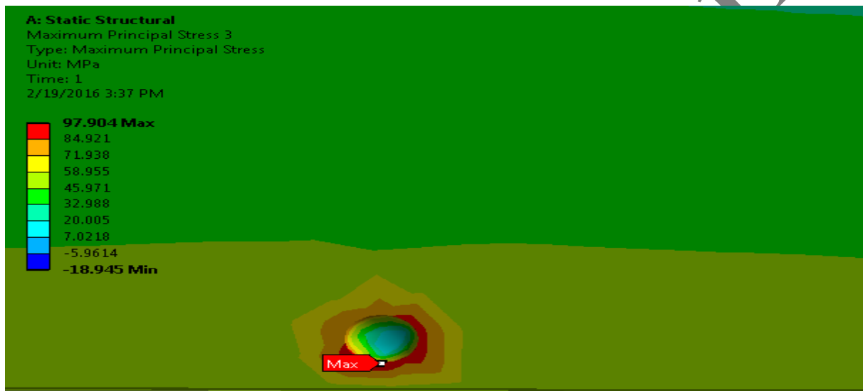
Fig. 3.6 Maximum Principal Stress in the Full Model with Void
