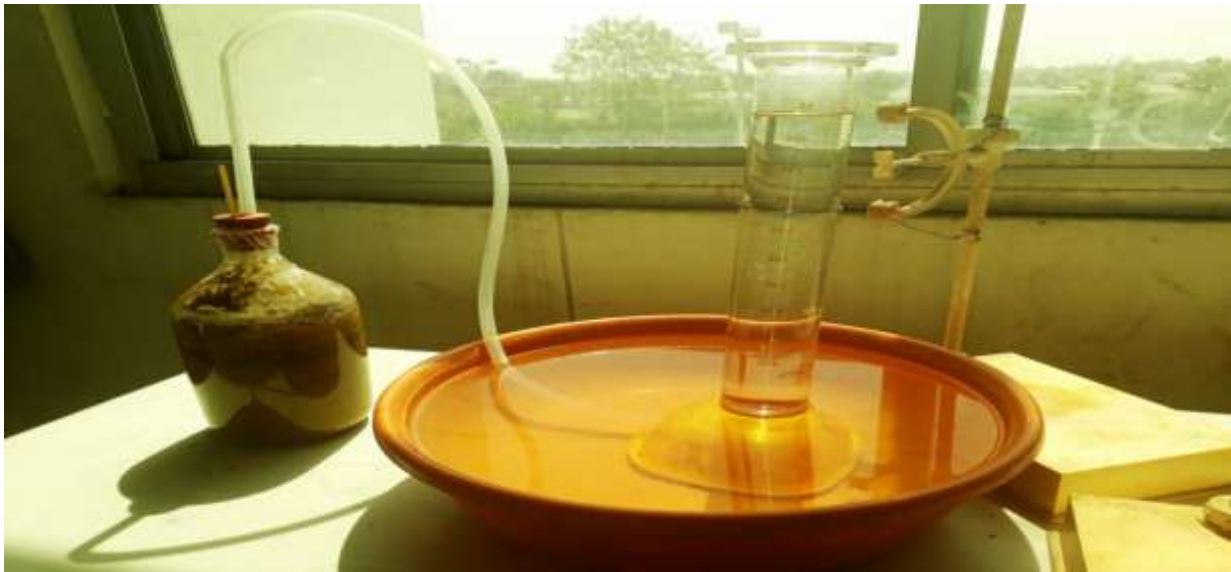
Fig. 3.2 A Kitchen Waste Biogas Plant
