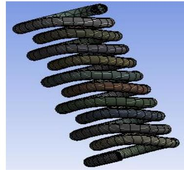
(c) Open-end variable outer diameter coil spring
