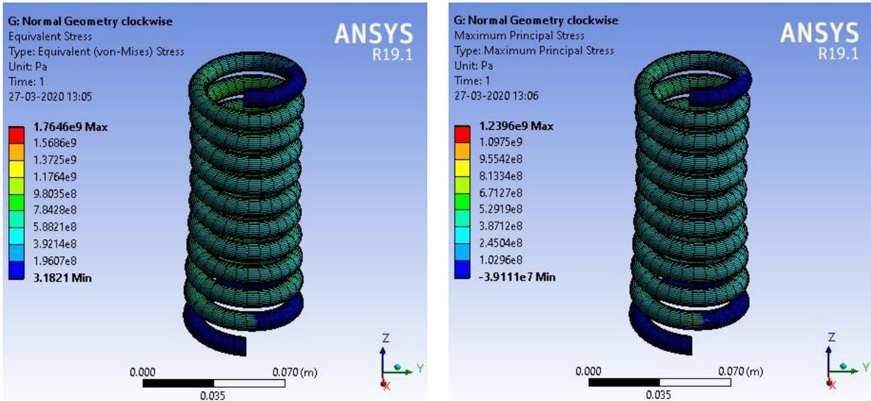
(a) Open-End Cylindrical Coil Spring
