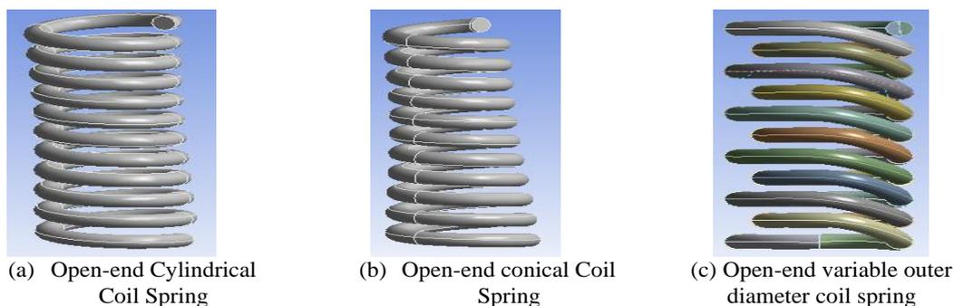
**Fig. 3.1 Various Geometrical Design of Coil Spring**
