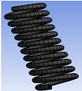
(a) Open-end Cylindrical Coil Spring
