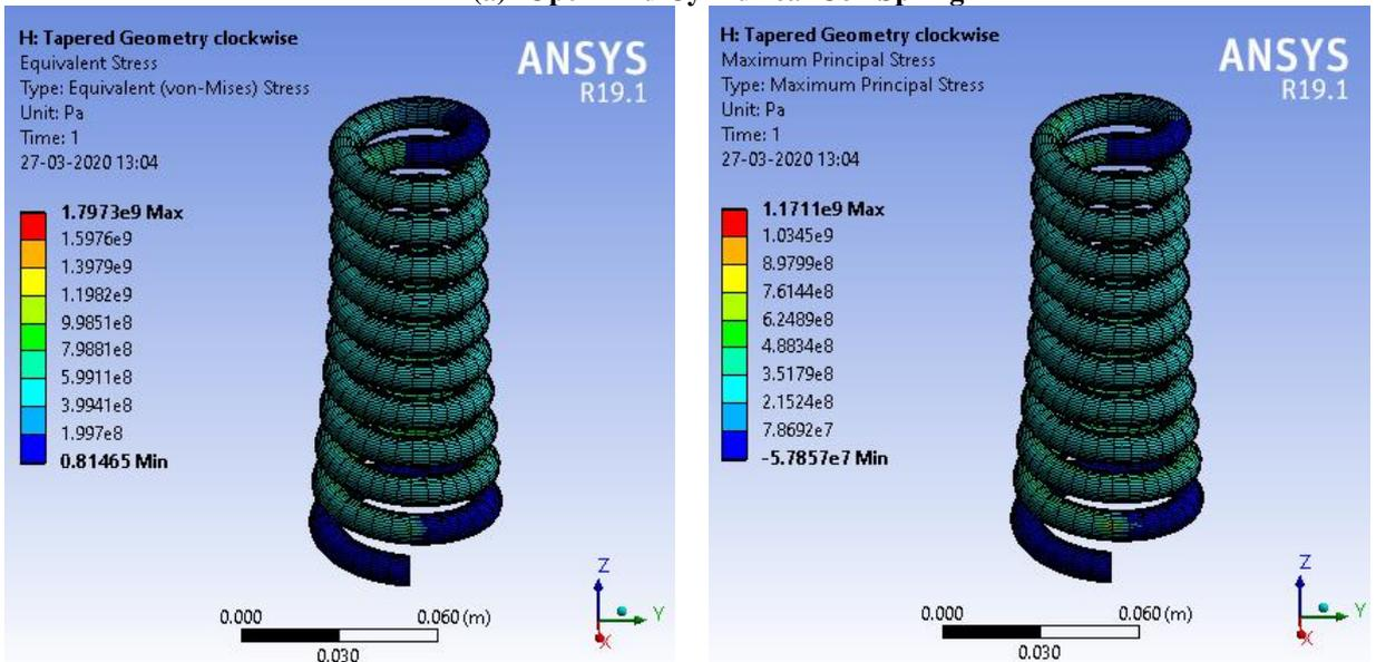
(b) Open-End Conical Coil Spring
