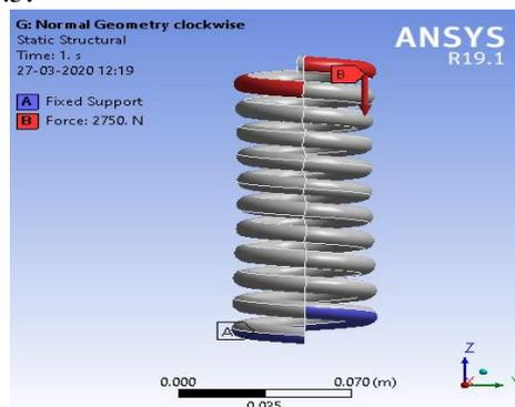
**Fig. 3.3 Boundary Condition on the Coil Spring for the Analysis**
