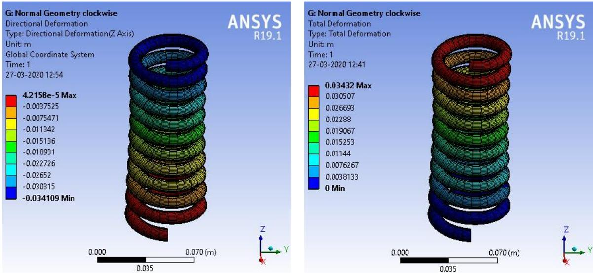
(a) Open-End Cylindrical Coil Spring
