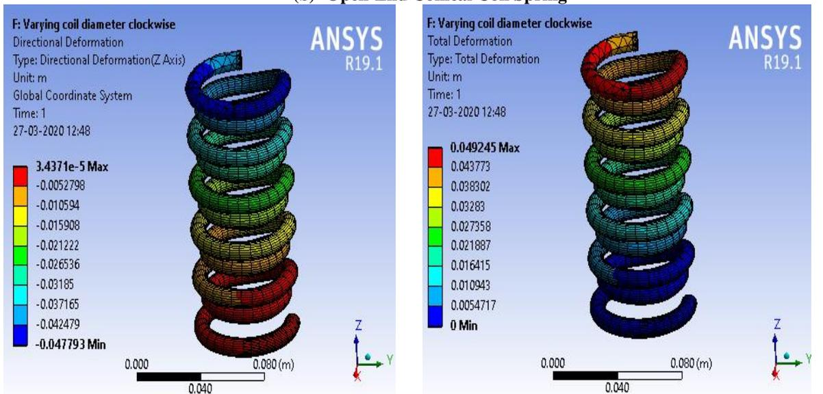
(c) Open End Variable Outer Diameter Coil Spring
