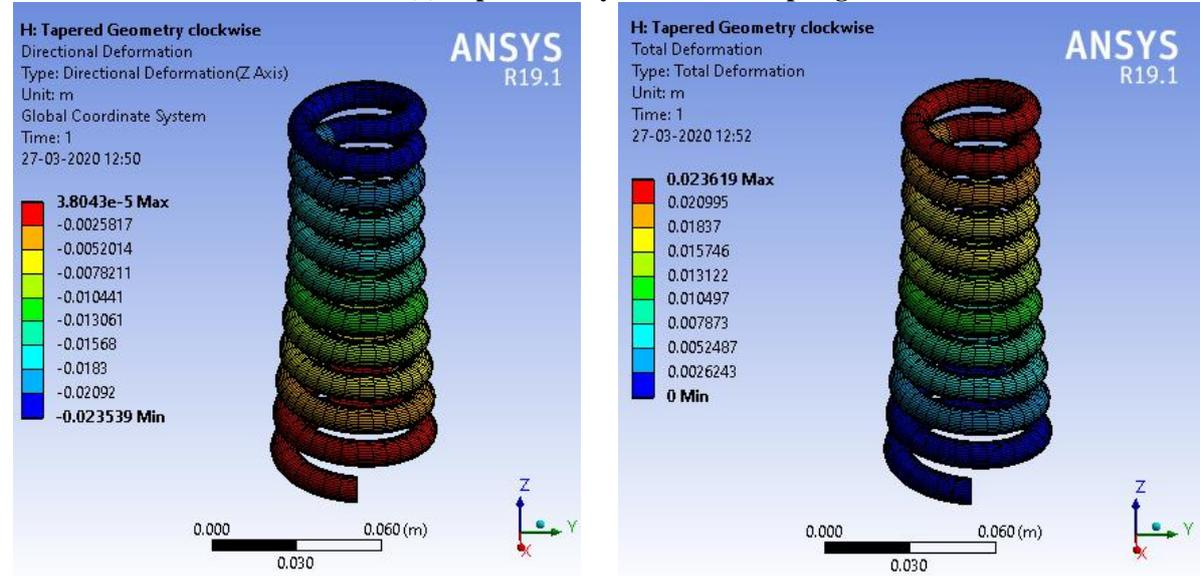
(b) Open-End Conical Coil Spring
