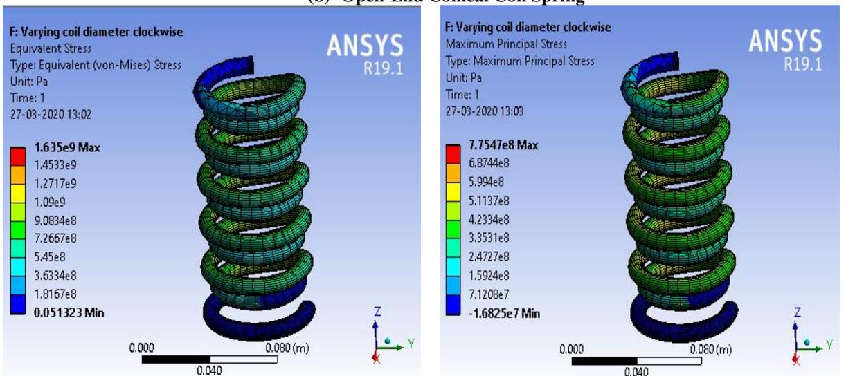
(c) Open End Variable Outer Diameter Coil Spring
