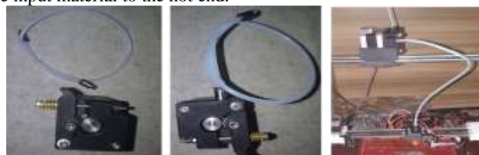
Fig. 2.10 PTFE Tube Teflon is Attached to the Static Part by 2xPneumatic Connector
