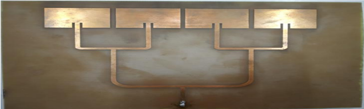
Fig. 3.11 Fabricated 2X2 Rectangular Array Antenna
