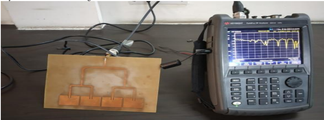
Fig. 3.12 Testing of 2X2 Rectangular Array Antenna using VNA
