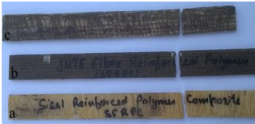
Fig. 3.1 Tested Tensile Samples (a) Sisal composite, (b) Jute compo-site, (c) Hybrid composite
