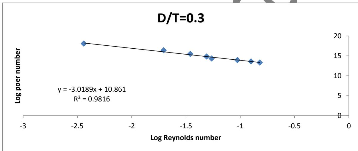
Fig. 3.3 Relation between log  $N_p$  and log  $Re$  of fig jam at 85°C
