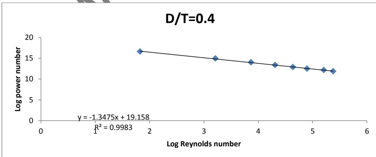
Fig. 3.4 Relation between log  $N_p$  and log  $Re$  of fig jam at 85°C
