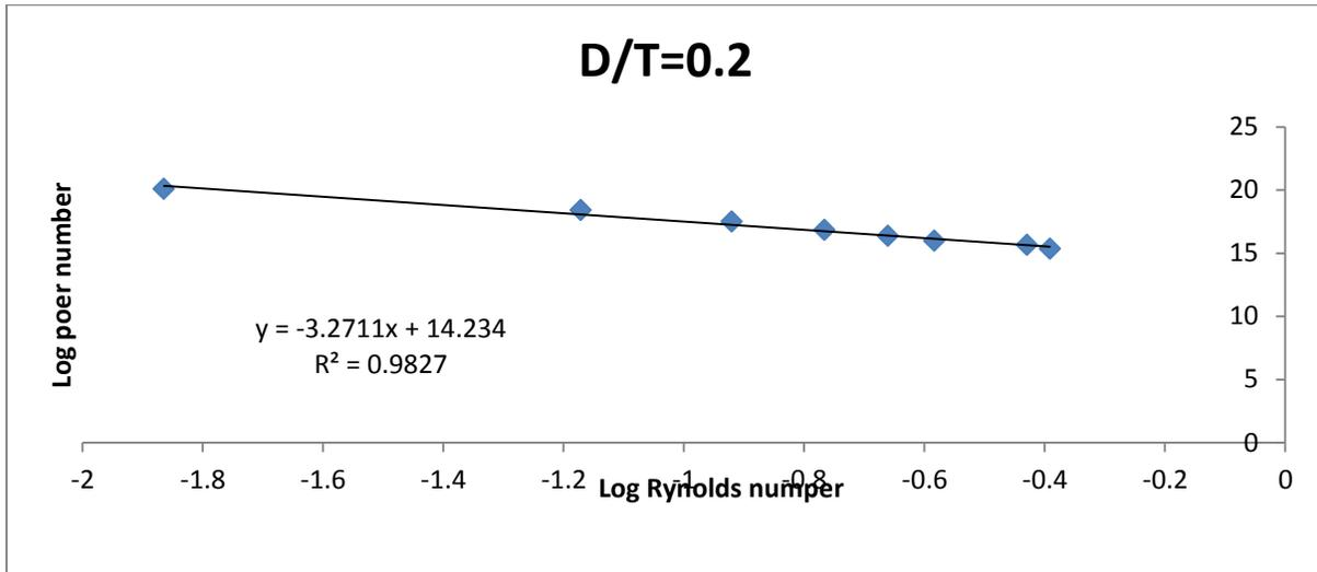
Fig. 3.2 Relation between log  $N_p$  and log  $Re$  of fig jam at 85°C
