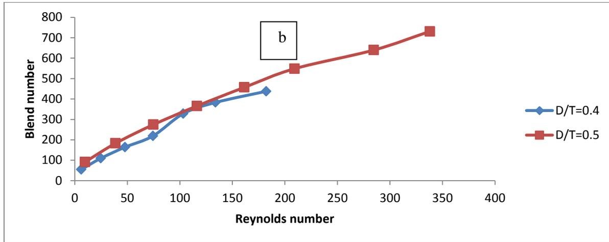
Fig. 3.6 Blend number ( $N_B$ ) as function of Re at different D/T ratios
