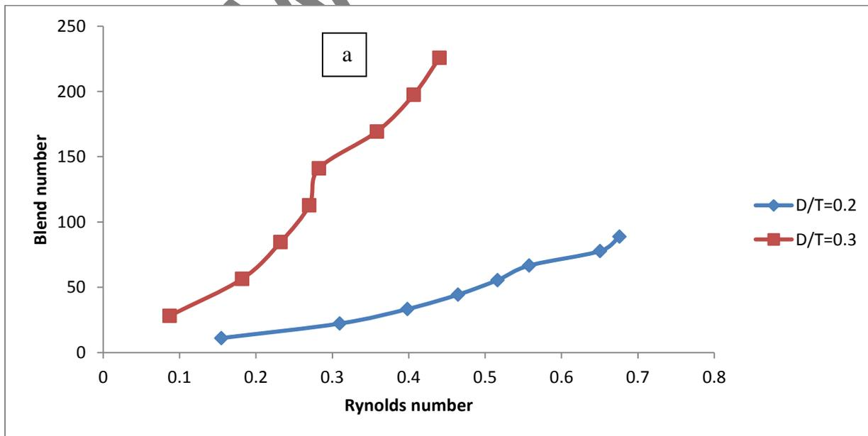
**Fig. 3.6 Blend number ( $N_B$ ) as function of  $Re$  at different D/T ratios**
