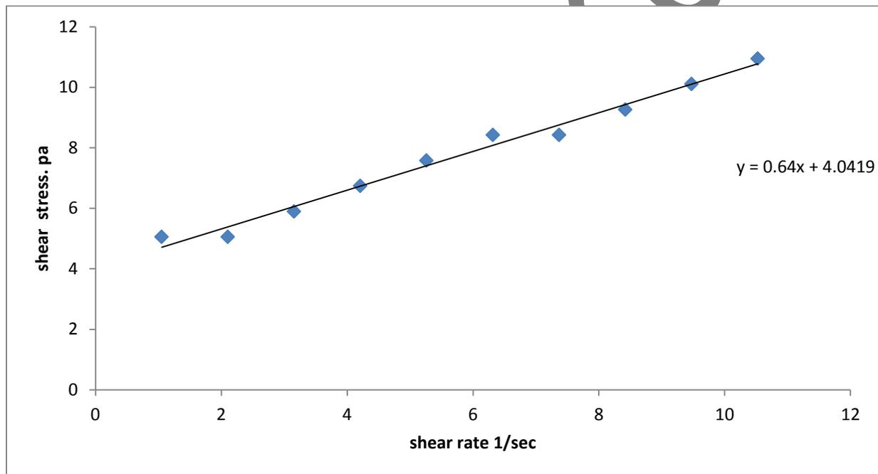
Fig. 3.1 Relation between Shear Stress and Shear Rate at 85 °C of 65 wt% Fig Jam
