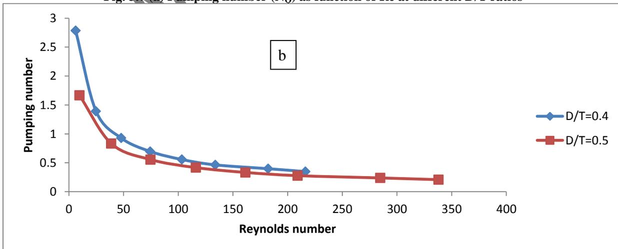
Fig. 3.7 (b) Pumping number ( $N_Q$ ) as function of Re at different D/T ratios
