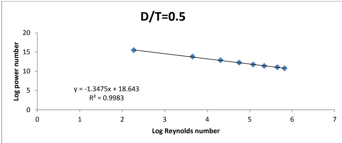
**Fig. 3.5 Relation between  $\log N_p$  and  $\log Re$  of fig jam at  $85^\circ\text{C}$**
