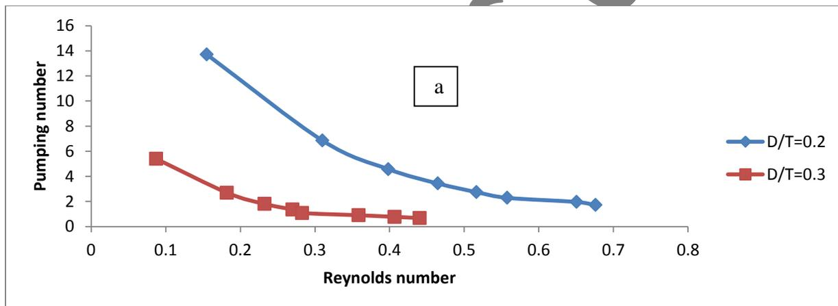
Fig. 3.7 (a) Pumping number ( $N_Q$ ) as function of Re at different D/T ratios
