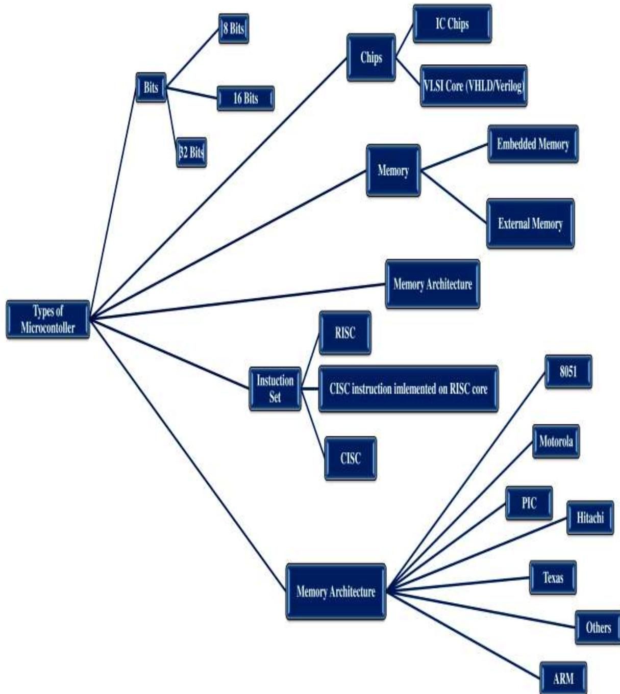
**Fig. 2.1 Classification of Microcontroller**
