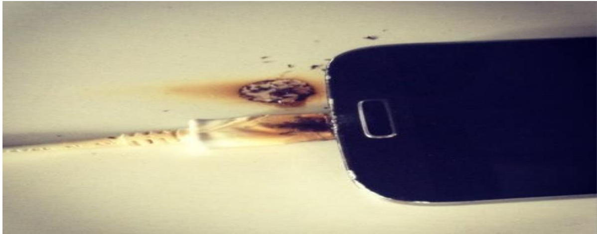
Fig. 3.1 Damaged Smartphone Due to Overcharging
