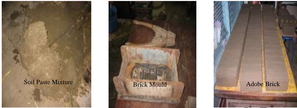
Fig. 3.2 Preparation Steps of Adobe Brick
