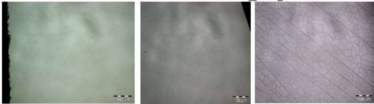
Fig. 3.1 Optical Images of a:SiC-H thin films (a) Annealed at 450 °C (b) Annealed at 650 °C (c) Annealed at 850 °C
