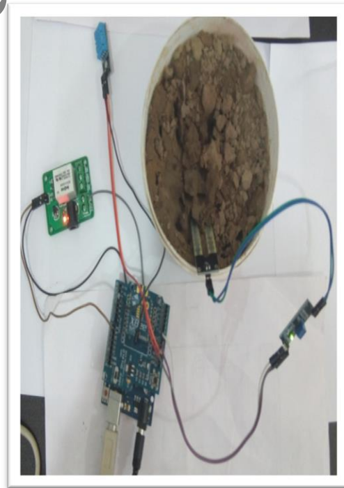
Fig 3.4 Testing of Soil Moisture Sensor and Relay
